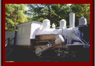
A Climax locomotive is a type of geared steam locomotive in which the two steam cylinders are attached to a transmission located under the center of the boiler. This transmits power to driveshafts running to the front and rear trucks.
