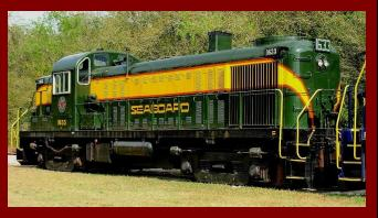
The American Locomotive Company (ALCO) manufactured produced 1,418 RS-3 locomotives from May 1950 to 1956. Slightly more powerful than its predecessor, the RS-2, it boasted a 1,600 HP 12-cylinder diesel-electric engine with a tractive effort of 61,755 pounds. Intended for road-switching duties, its primary competitors were the EMD GP7 and GP9, Fairbanks-Morse's H-15-44 and H-16-44, and Baldwin's DRS-4-4-15 and AS-16
