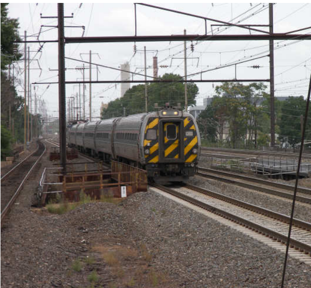
Above: On the platform, looking south. The old Pennsy position light signals are still in use, but have been recently relamped for 2 colored lights instead of three amber. Union Tower, beyond, still protects Union Interlocking, the junction of the Northeast Corridor and the North Jersey Coast Line. Below left: Amtrak Metroliner control cab 9638 leads a rare consist pushed by an AEM-7. Lower right: NJ Transit ALP-46 No. 4601 pauses it's train of bi-levels on Track 6 on its way to the Amboys and Bay Head. NJ Transit operates its trains push-pull fashion, typically with locomotives leading outbound from Penn Station. Today, though, many trains seem to deviate from this norm.
