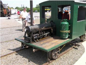
Top left: Seaboard Air Line 2-10-0 Russian No. 544, built by ALCO in 1918. Upper right: NS GP-59 4610. Lower left: NS SD70M-2 No. 2720 reflected in the windows of the Back Shop, which is still closed awaiting renovation. Lower right: A Steamer Speeder! Among the half dozen motor cars that provided short rides was this propane-fired steamer. The "live steam" locomotive has belts looping the driver axels that propel the car. It was also the quietest one of the bunch.
