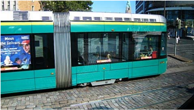
These two pictures show joints required when making the sharp curves
